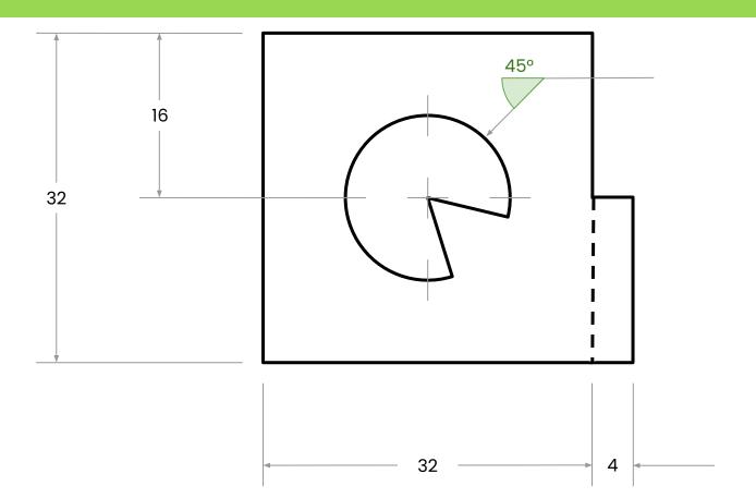
9. Dimensions used to identify the **radius** of a circle are preceded by an **R**. They are preceded by the symbol  $\circ$  or the letters **DIA** when they indicate the diameter.
