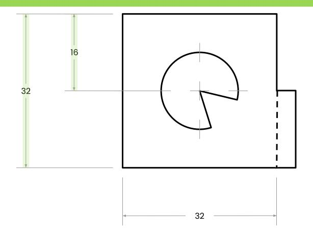
7. If the space between the extension lines is too small, the **arrows** go on the **outside**. The **dimension** can go **inside** or **outside** the extension lines, depending on how much space there is.
