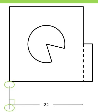
3. There is a gap of **at least 10 mm** between the side of an object and the dimension lines or between two dimension lines.
