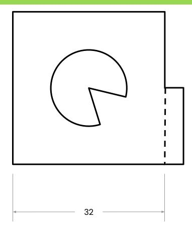
2. The **extension lines** are **perpendicular to the dimension lines** and start **2 mm away** from the side of the object. They extend **2 mm beyond** the ends of the dimension lines.
